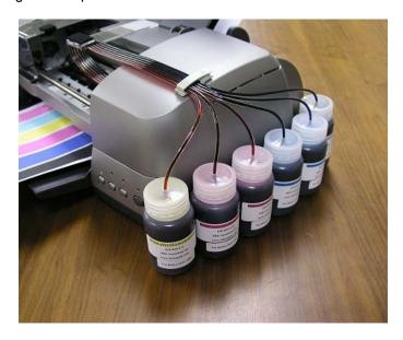
Insert the tubing into the tube clip and close it until it snaps shut. Don't pinch any of the tubes.
